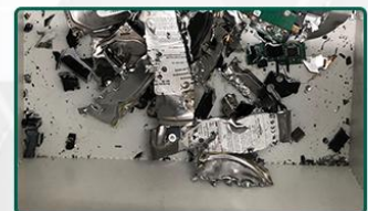
HD2000 H4 Hard disk shredder Shredding capacity: >200 pcs/hr Shredding particle size: 18mm*random
