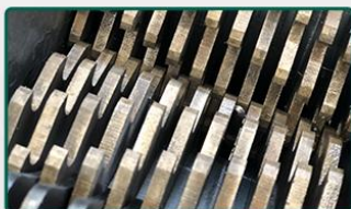
HD1000 Office use small HDD shredder Shredding capacity: 60 pcs/hr Shredding particle size: 20mm*random
